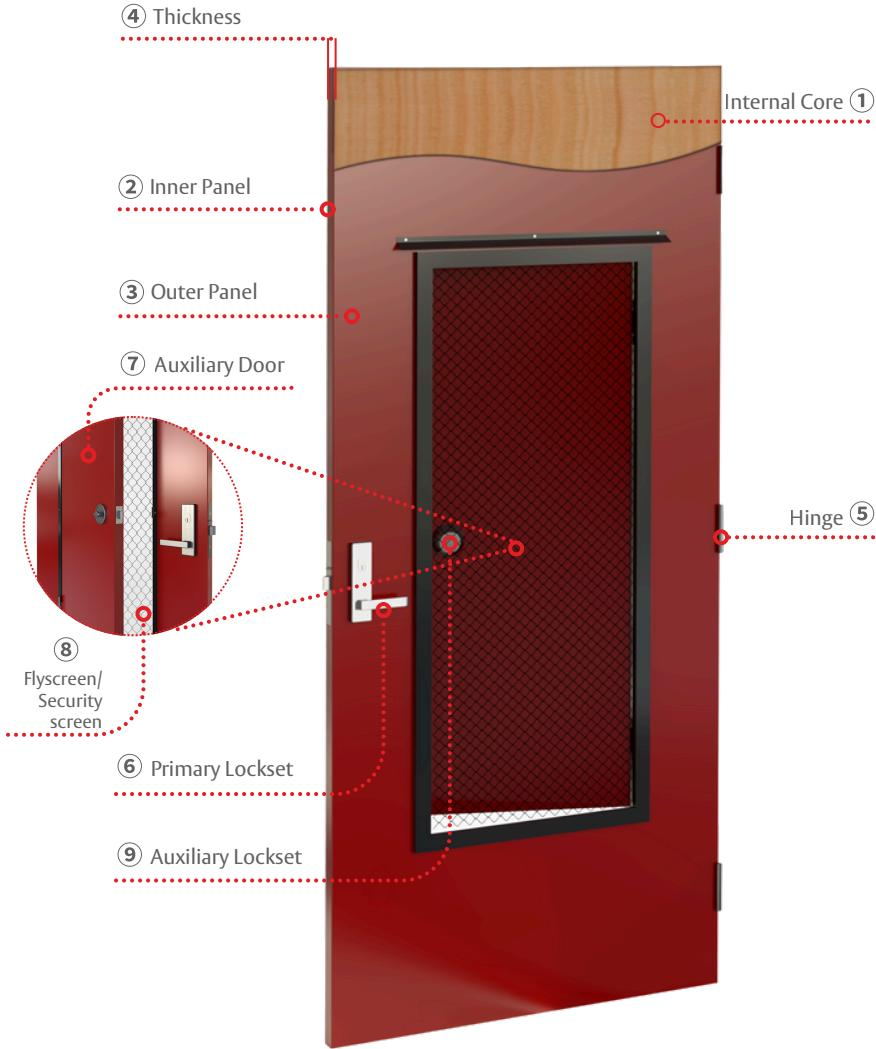
The **Duo metal clad solid core door**, integrated with an auxiliary door and an auxiliary door mesh, offers reversible handing, operates inward or outward, and is available in a full range of sizes in single-leaf configuration.
