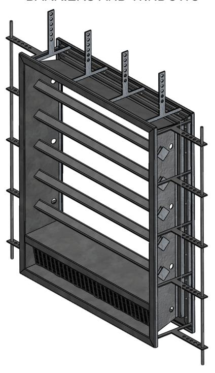
HIGH SECURITY STYLE BARRIERS AND WINDOWS DESIGNED AND MANUFACTURED IN-HOUSE OR TO ARCHITECHTURAL SPECIFICATIONS. T STRAPS, REO BAR, AND BRACING CAN ALL BE ADDED FOR PRE CAST INSTALATION
