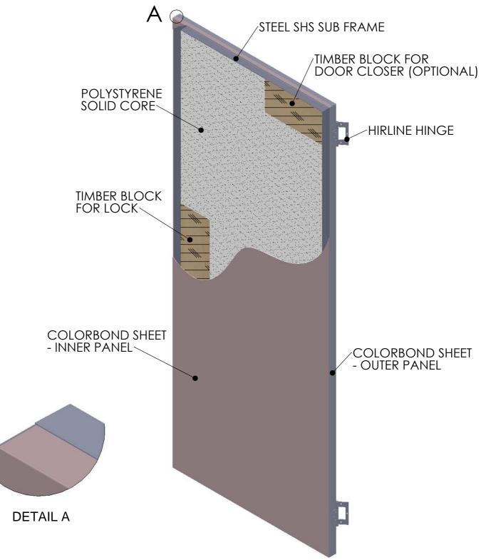
THE EDGE TREATMENT OF A SECURITY 1 DOOR GIVES YOU THE FINISH OF A TIMBER DOOR AND HIGH SECURITY OF A MEDIUM STEEL CLAD DOOR
