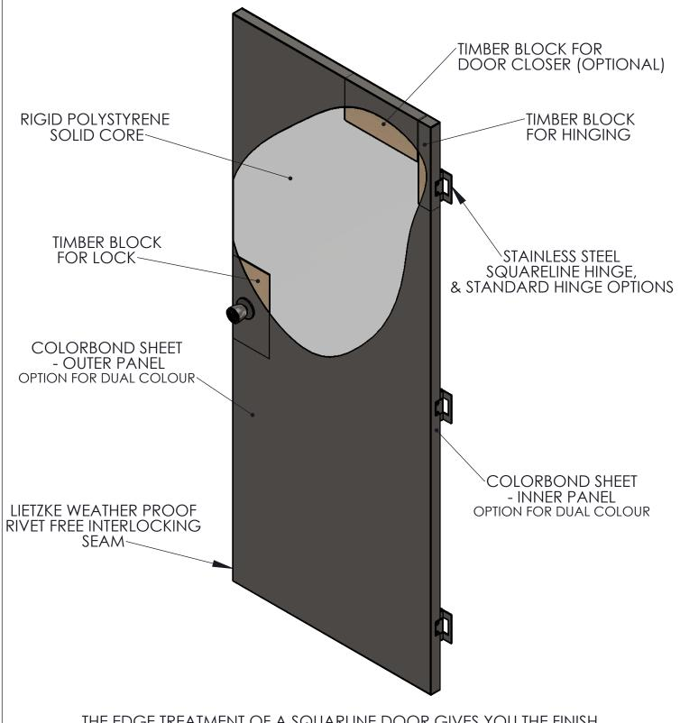
THE EDGE TREATMENT OF A SQUARLINE DOOR GIVES YOU THE FINISH OF A TIMBER DOOR AND THE SECURITY OF A METAL CLAD DOOR
